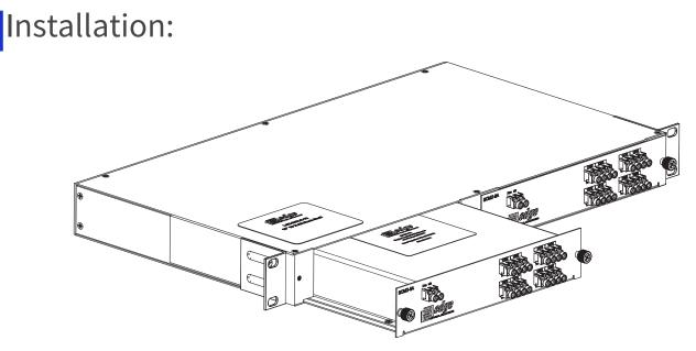
In order to install CWDM LGX Module in 19" rack, please order 19" 1U sub-rack supporting up to two LGX modules. Product code LGX-RCK-2-1U.
